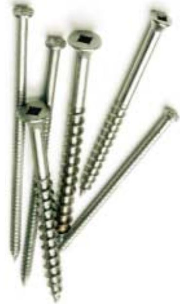
To prevent unsightly stains, only corrosion-resistant hot-dipped galvanized, aluminum, or stainless steel fasteners should be used with cedar. Stainless steel is the best choice.
